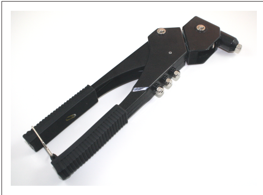
FIGURE 2-10. Hand-operated blind rivet installation tool
