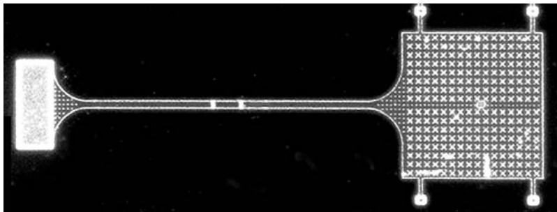
FIGURE 3.3 A tensile specimen fixed at the left end with a free grip end at the right end. (Reprinted with permission from Sharpe, W.N., Jr., and Jackson, K. [2000] Microscale Systems: Mechanics and Measurements Symposium, Society for Experimental Mechanics , pp. ix–xiv.)
