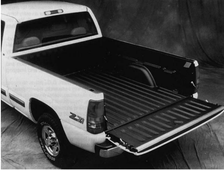
FIGURE 1.7 One-piece cargo box for a pickup truck made by the SRIM process.
