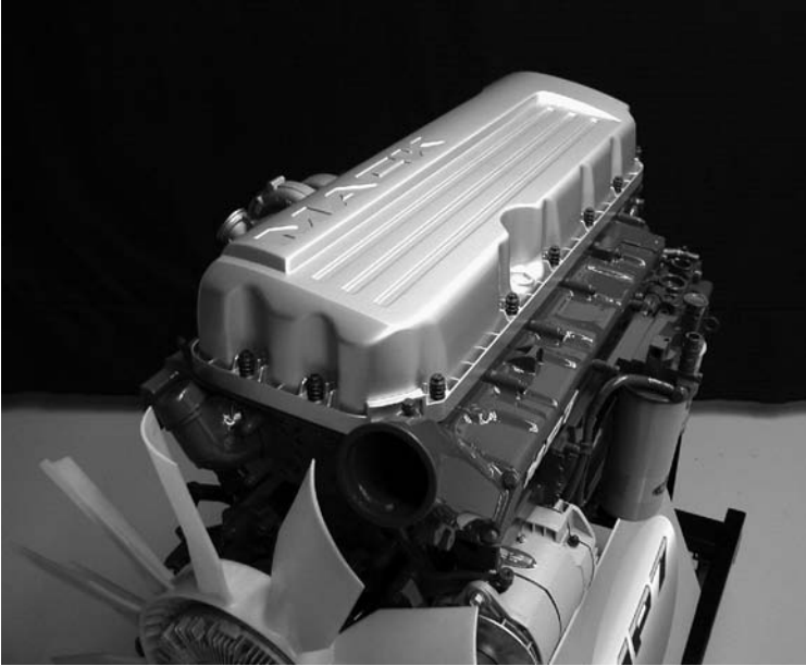
FIGURE 1.6 Compression-molded SMC valve cover for a truck engine. (Courtesy of Ashland Chemicals and American Composites Alliance. With permission.)
