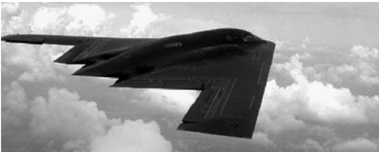
FIGURE 1.1 Stealth aircraft (note that the carbon fibers in the construction of the aircraft contributes to its stealth characteristics).
