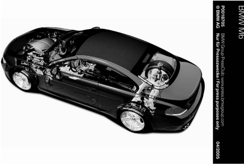
FIGURE 1.8 Carbon fiber-reinforced epoxy roof panel in BMW M6 vehicle. (Photograph provided by BMW. With permission.)
