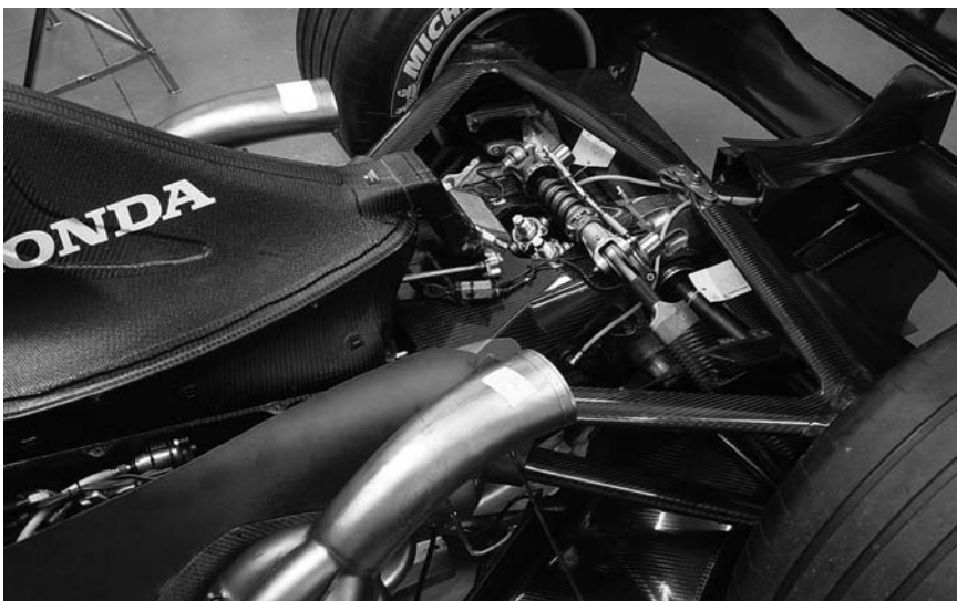
FIGURE 1.9 Carbon fiber-reinforced epoxy suspension and gear box in a Formula 1 race car. (Courtesy of Bar 1 Formula 1 Racing Team. With permission.)
