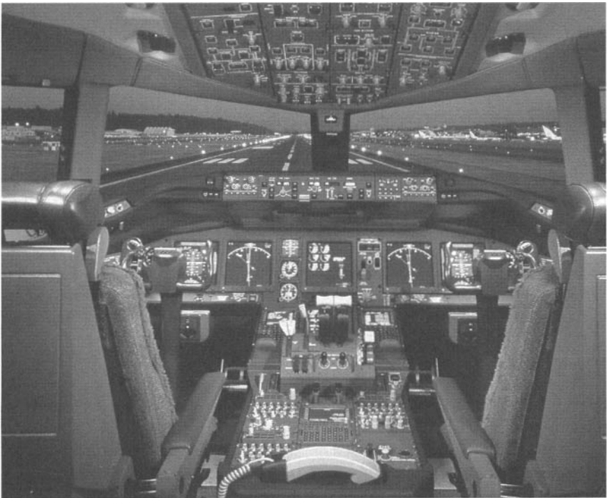
FIG. 1.3 The Boeing 777-300 flight deck: The newest member of the 777 family is a large, modern commercial air carrier. The 777 flight deck illustrates the use of large multipurpose displays to efficiently convey a great deal of information to the crew. (Courtesy of the Boeing Company)
