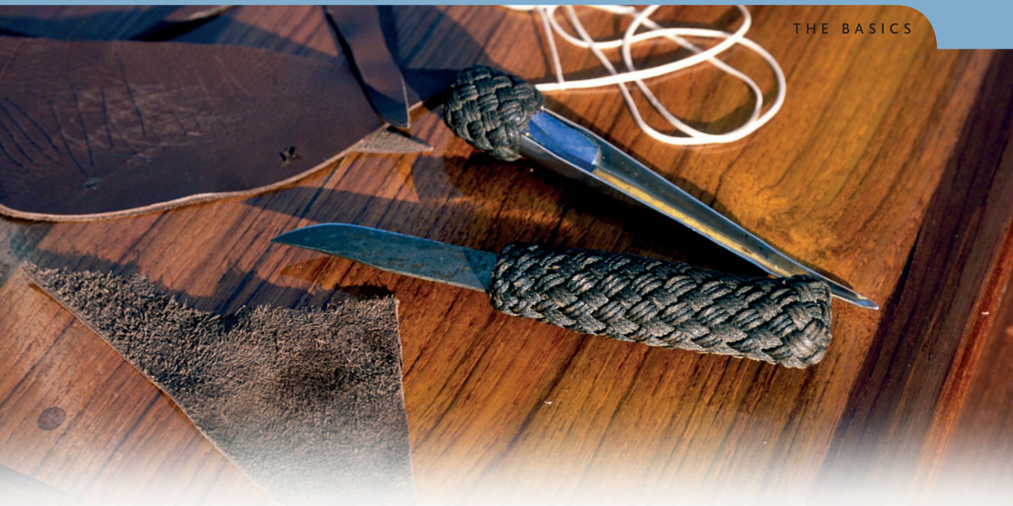
Above A rigger's knife and marlinspike (or, strictly, a fid). You don't need much else for 90 per cent of the knots in this book.
