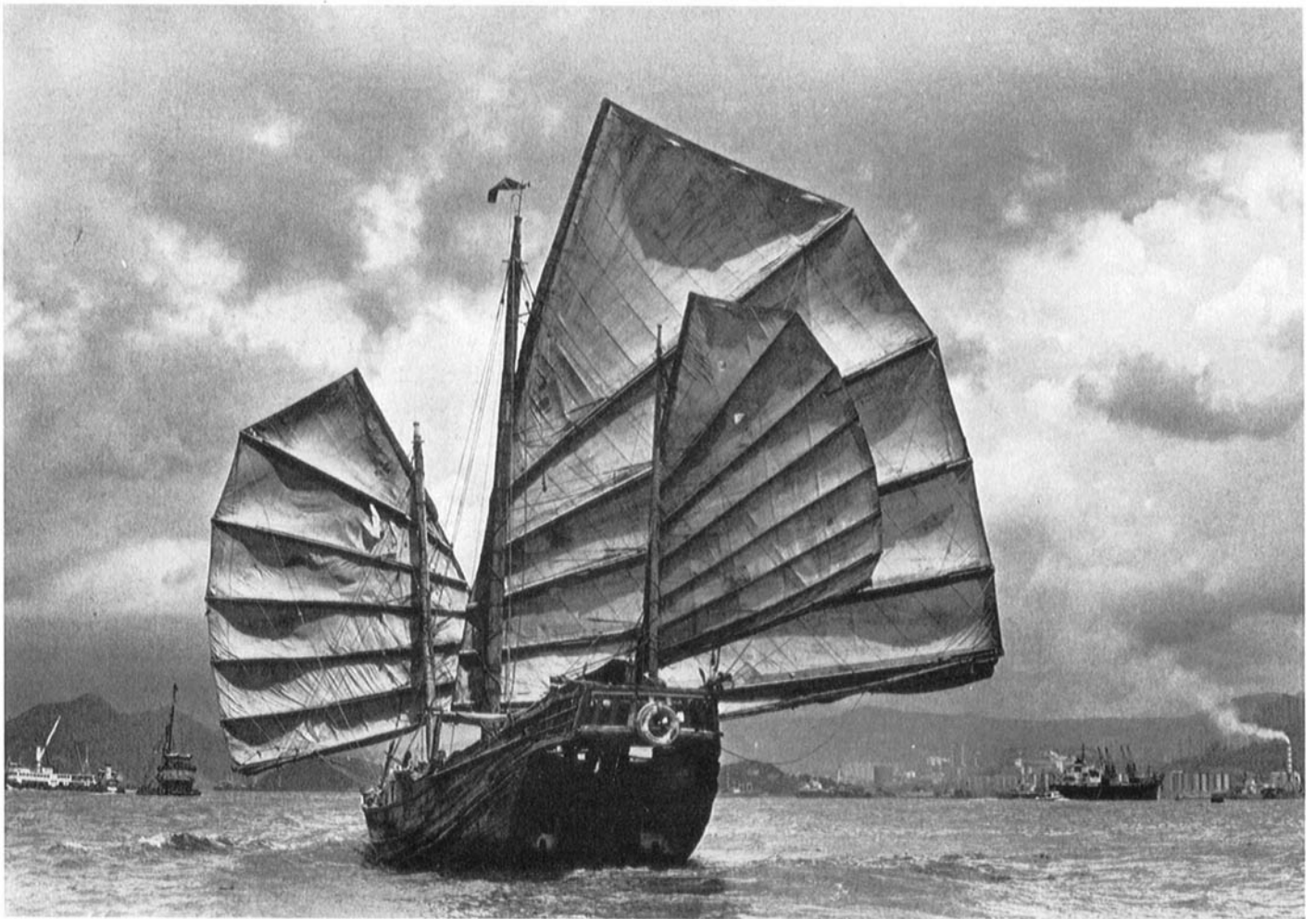
A large Chinese Junk running goosewinged. Note the huge mainsail and the different balance of the sails and their design. (Photo: South China Morning Post Ltd)
