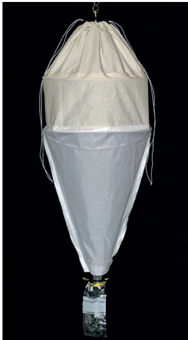
Figure 43. Collapsible Berlese funnel for extracting small beetles and other arthropods from litter.
