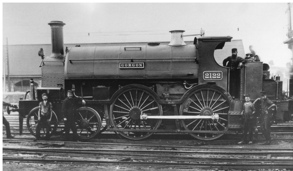
4-4-0ST 2122 Gorgon built in 1866 and which lasted to the end of the broad gauge in 1892, seen here c1890. (GW Trust)
