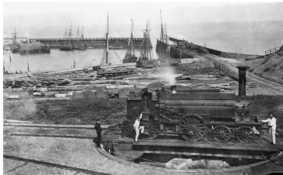
Bristol & Exeter broad gauge 4-4-0T, No.74, built by Vulcan, 1867, at work on the docks at Watchet in north Somerset, an early photograph thought to be at the end of the 1860s or early 1870s. (F.K. Davies/John Hodge Collections)
