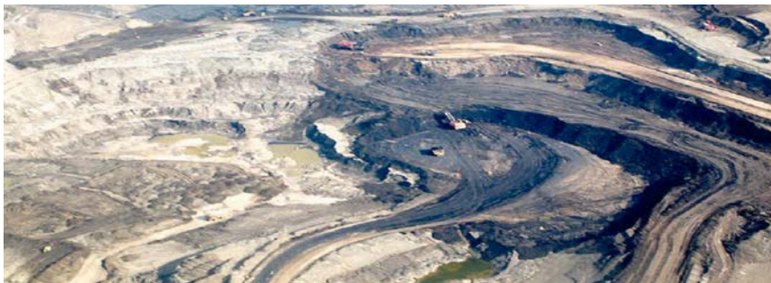
FIGURE 1.6 Surface mining for recovery of bitumen.
