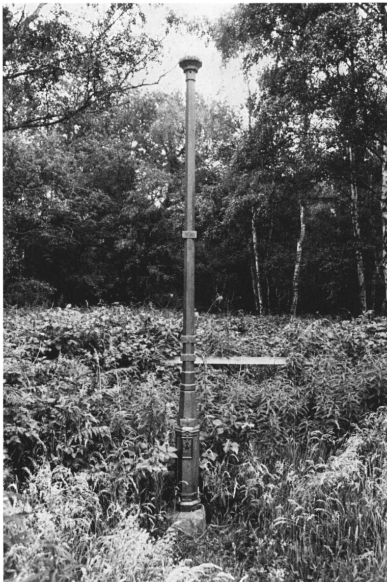
FIGURE 7 The Holme Fen post, Fenland, England. The post was driven into bedrock under Fenland peats in 1848, with its top exactly at ground level. The height now seen (over 3 m) represents shrinkage (not cutting) of the peat due to drainage of the area.
