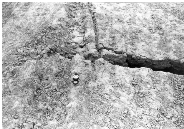
Figure 2.36 Detail of the rut displaced due to creep shown in Figure 2.35.
