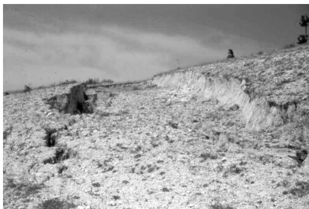
Figure 2.38 Secondary normal ground deformations in the form of grabens forming in the upthrust block of marls as a result of the El Asnam earthquake ( M_s 7.2) in Algeria of 10 October 1980. These secondary features give the impression of normal surface faulting produced in an earthquake of thrust mechanism.
