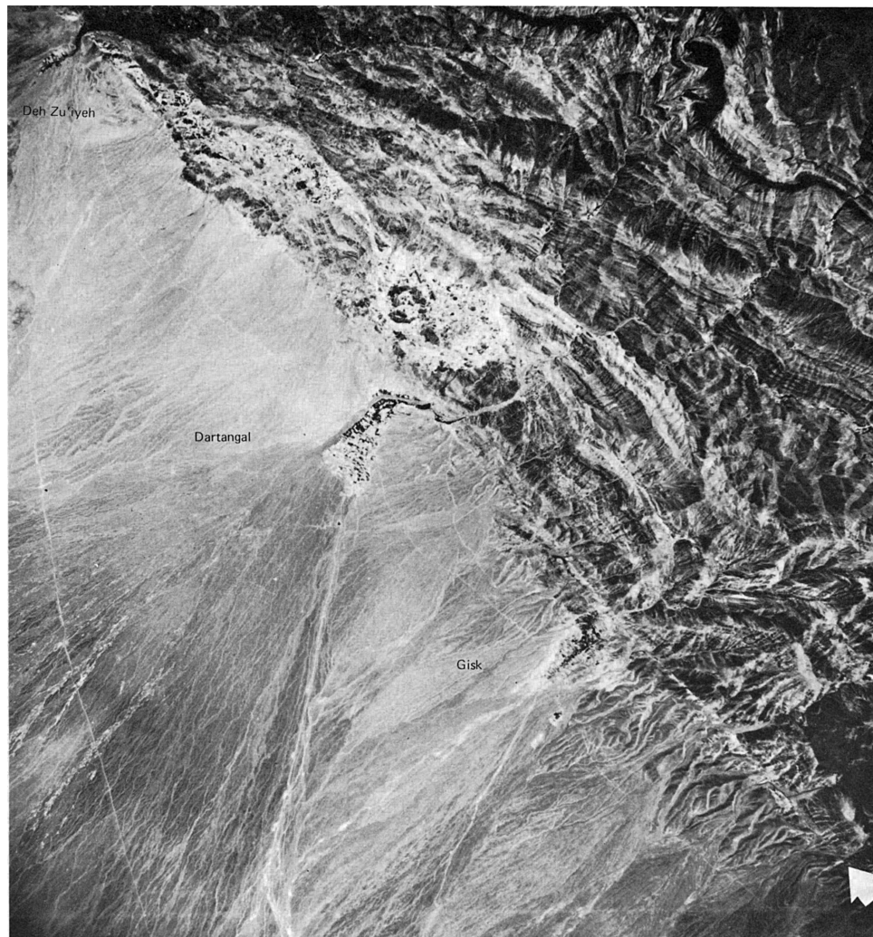
Figure 2.5 An aerial view of the Kuhbanan fault associated with the Gisk earthquake of 19 December 1977 of M_S 5.9. The village in the centre is Dartangal. (Scale: the distance between Dartangal and the tip of the arrow in the right-hand corner of the figure, which marks the fault, is 8 km.)
