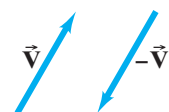
FIGURE 3-7 The negative of a vector is a vector having the same length but opposite direction.
