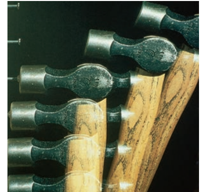
FIGURE 4–7 A hammer striking a nail. The hammer exerts a force on the nail and the nail exerts a force back on the hammer. The latter force decelerates the hammer and brings it to rest.
