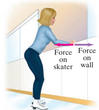
FIGURE 4–9 An example of Newton’s third law: when an ice skater pushes against the wall, the wall pushes back and this force causes her to accelerate away.
