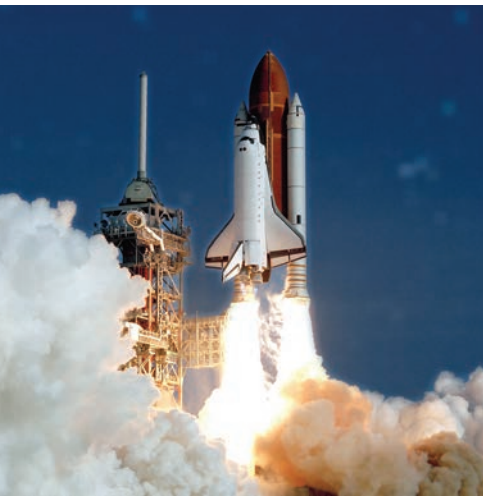
FIGURE 4–10 Another example of Newton’s third law: the launch of a rocket. The rocket engine pushes the gases downward, and the gases exert an equal and opposite force upward on the rocket, accelerating it upward. (A rocket does not accelerate as a result of its expelled gases pushing against the ground.)
