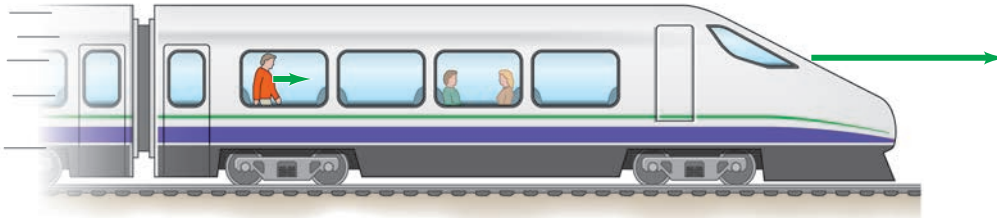
FIGURE 2–2 A person walks toward the front of a train at 5 km/h. The train is moving at 80 km/h with respect to the ground, so the walking person’s speed, relative to the ground, is 85 km/h.
