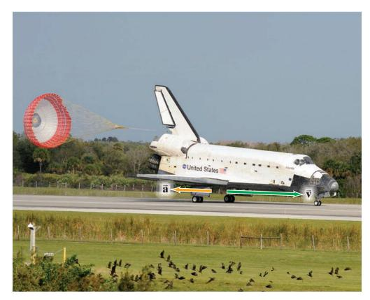
The space shuttle has released a parachute to reduce its speed quickly. The directions of the shuttle's velocity and acceleration are shown by the green  $(\vec{\mathbf{v}})$  and gold  $(\vec{\mathbf{a}})$  arrows.
