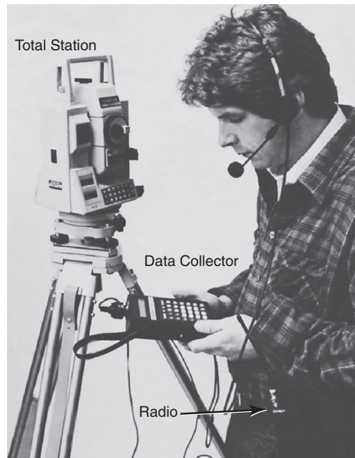
FIGURE 1.6 Sokkia total station.
