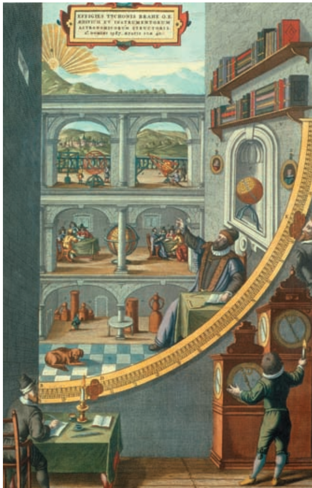
FIGURE 15 Tycho Brahe in his naked-eye observatory, which worked much like a giant protractor. He could sit and observe a planet through the rectangular hole in the wall as an assistant used a sliding marker to measure the angle on the protractor.
