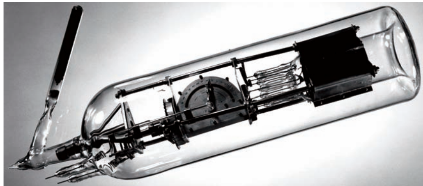
Figure 4 Davisson and Germer's original electron diffraction apparatus, showing the mechanism for varying a sample's angle.
