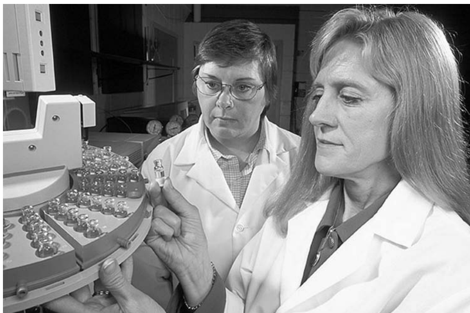
Figure 2 Dr. Pamela White, Dean of the College of Human Sciences at Iowa State University, is loading vials into the automatic injector of a gas chromatograph as she conducts an experiment on oils.
