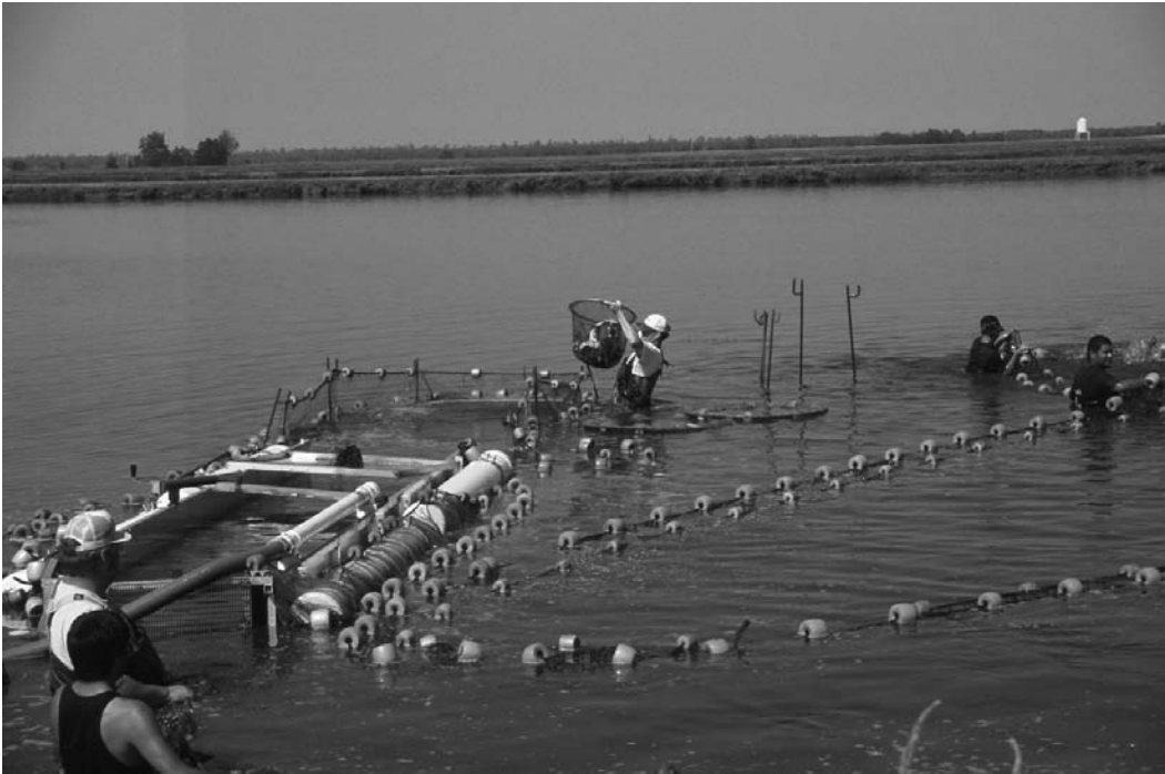
Figure 2 Researchers and fish farmers sample catfish to check the efficiency of a floating platform grader near Belzoni, Mississippi. (Courtesy of Agricultural Research Service.)
