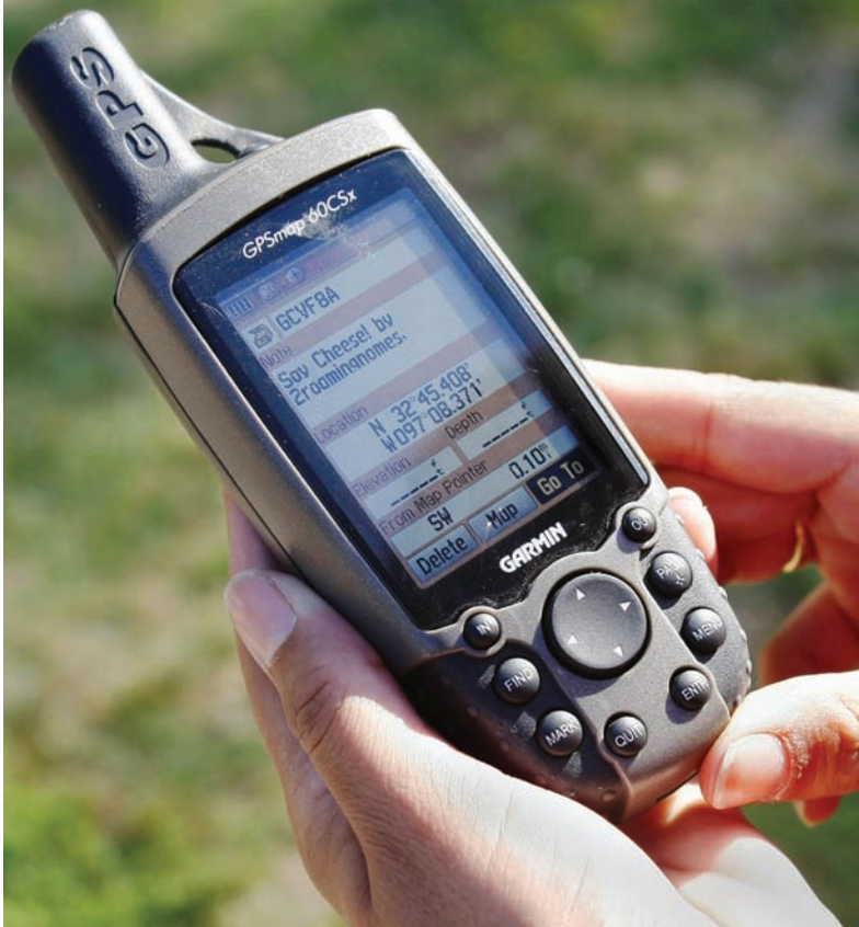
▲ Figure 18 A handheld GPS receiver. It receives signals sent by the network of Global Positioning System satellites, calculating its position anywhere in the world to within 10 meters (33 feet).
