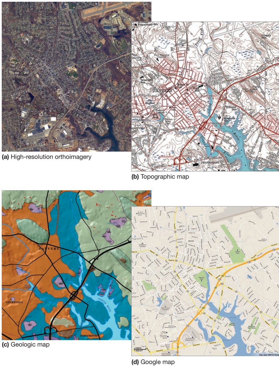
▲ Figure 1 Different types of maps convey different kinds of information about the landscape, as shown in these four maps of a region near Salem, Massachusetts. (a) High-resolution orthophoto imagery (original scale 1:24,000). (b) Topographic map with elevation contour lines (original scale 1:24,000). (c) Geologic map showing rock types: orange = coarse glacial deposits; blue = glaciomarine deposits; green = glacial till; lavender = swamp deposits (original scale 1:50,000). (d) Google™ Map showing streets and highways.
