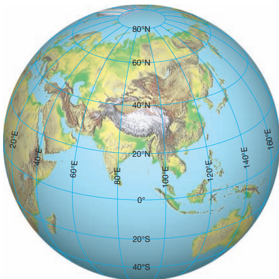
▲ Figure 10 An orthographic planar projection showing Earth as it would appear from space.
