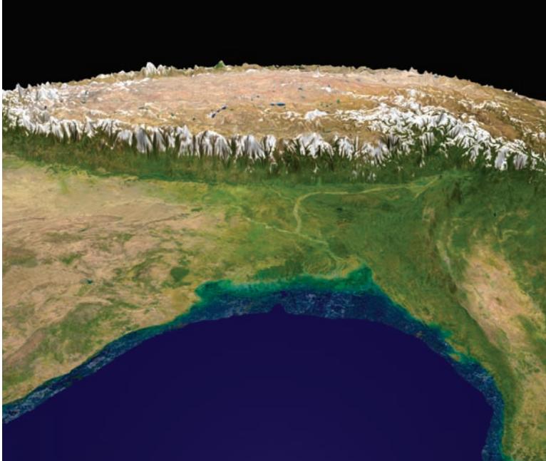
▲ Figure 29 This oblique view of Bangladesh and the Himalayas was created by configuring MODIS images from the Terra satellite over a 50-times vertically exaggerated digital elevation model of the topography.
