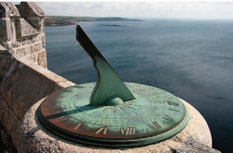
◀ Figure 30 A typical sundial. The edge of the vertical gnomon slants upward from the dial face at an angle equal to the latitude of the sundial, pointing toward the North Pole in the Northern Hemisphere and the South Pole in the Southern Hemisphere. As the Sun appears to move across the sky during the course of a day, the position of the shadow cast by the gnomon changes. The time shown in this photograph of a sundial in Cornwall, United Kingdom, is about 11:00 A.M.
