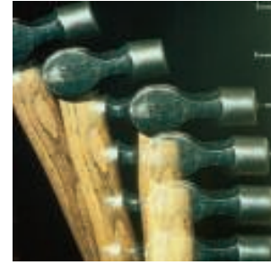
FIGURE 7 A hammer striking a nail. The hammer exerts a force on the nail and the nail exerts a force back on the hammer. The latter force decelerates the hammer and brings it to rest.
