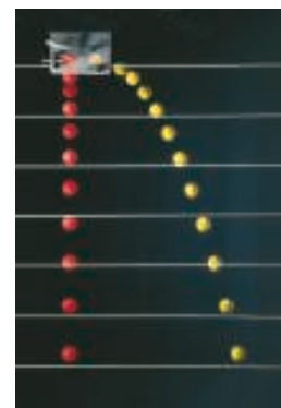
FIGURE 21 Multiple-exposure photograph showing positions of two balls at equal time intervals. One ball was dropped from rest at the same time the other was projected horizontally outward. The vertical position of each ball is seen to be the same at each instant.
