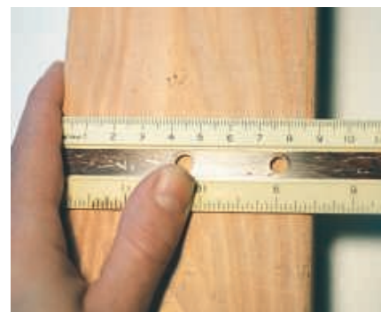
FIGURE 2 Measuring the width of a board with a centimeter ruler. The uncertainty is about \pm 1 mm.
