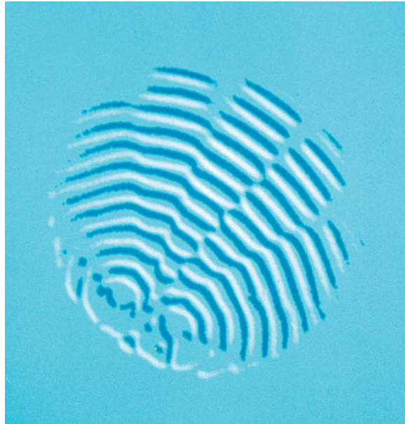
Fig. 1.4 The interference pattern produced by two vibrating sources in water.
