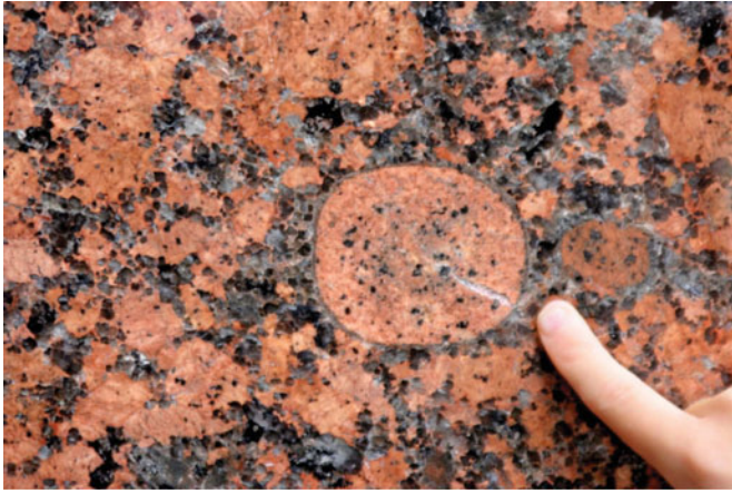
Figure 2.13 Rapakivi granite is one of the most common decorative building stones. It is shipped from quarries in southern Finland all over the world. Its characteristic texture is created by large rounded pink crystals of alkali feldspar rimmed by grayish-green plagioclase feldspar.
