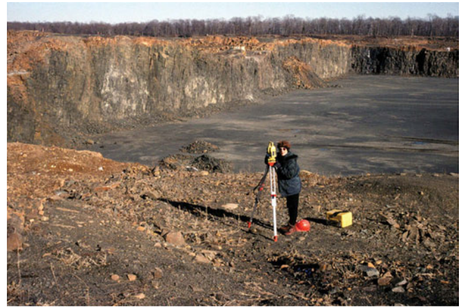
Figure 2.9 The active north face of Tilcon's North Branford quarry, Connecticut, where a thick basaltic lava flow is quarried for its extremely durable rock that is used as aggregate and mixed with asphalt to pave roads. This quarry produces 20 000 tons of crushed trap-rock aggregate per day.
