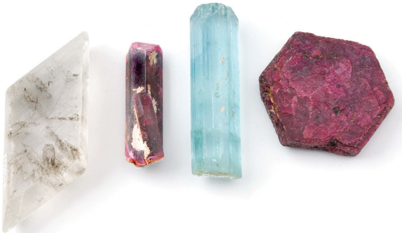
Figure 2.8 Examples of some very well-formed (euohedral) crystals. From left to right: a milky, translucent crystal of gypsum; a red crystal of tourmaline; a transparent, light blue crystal of aquamarine (a gem variety of the mineral beryl); and a red crystal of ruby (a gem variety of the mineral corundum).
