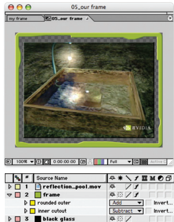
22 » FOR THE XFX VIDEO, WE CREATED SLIGHTLY FANCIER FRAMES WITH ROUNDED EDGES BY USING TWO MASK SHAPES.
