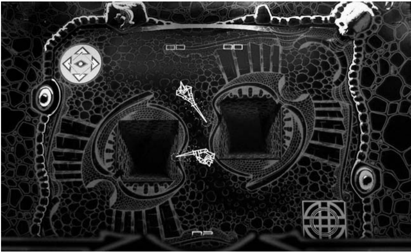
Figure 0.1 For the game Warrior (1979), static artwork was reflected over a vector display, an ancient illusion in the service of video games. (Photograph by Archer Maclean.)
