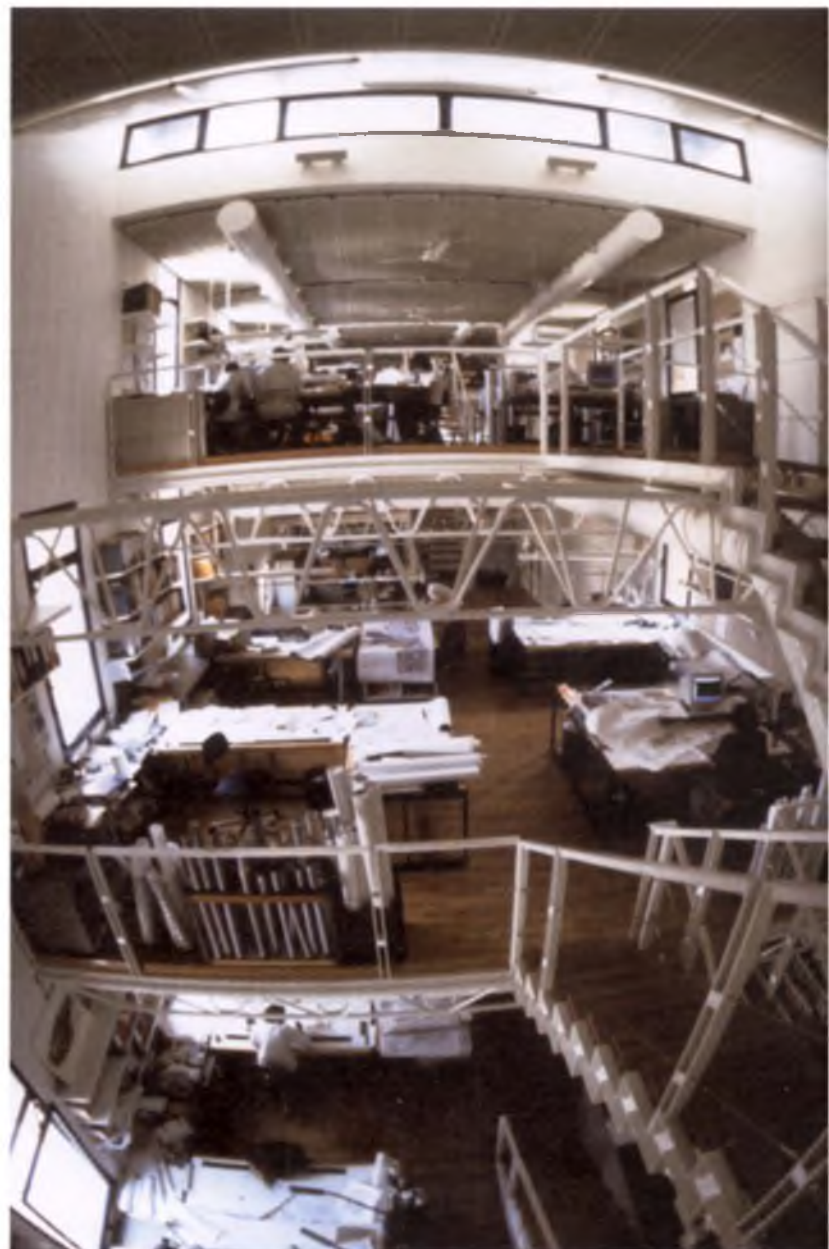
Δ The Architects Office in Athens is a good example of a building where facade window area has been reduced to a minimum size because of the climate, still achieving a bright work space near each window. The rest of the room benefits from ambient light admitted by a central roof monitor equipped with shading devices.
