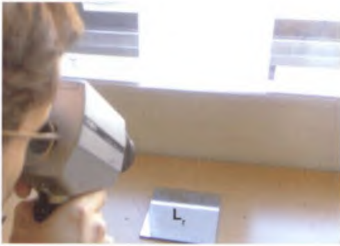
Δ On site determination of the specular reflectance ( \rho_s ) at a given angle: the luminance of the reflection ( L_r ) is compared to the luminance of the source of light ( L_s ), seen from the sample. \rho_s = L_r / L_s
