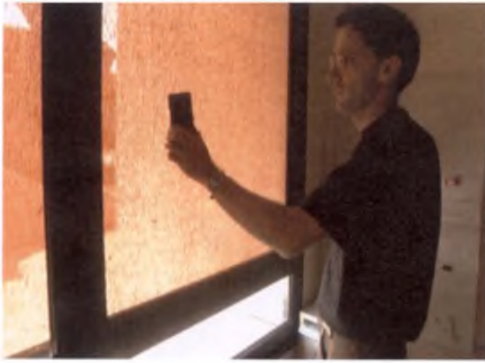
Δ Assessment of hemispherical - hemispherical transmittance of diffusing awnings. No direct sun beams should hit the window pane - overcast sky conditions preferred.
