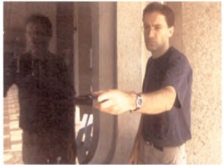
Δ Determination of the contribution of light reflections on the external ground. The luxmeter is oriented upward and downward to compare light coming from the upper and lower hemispheres.
