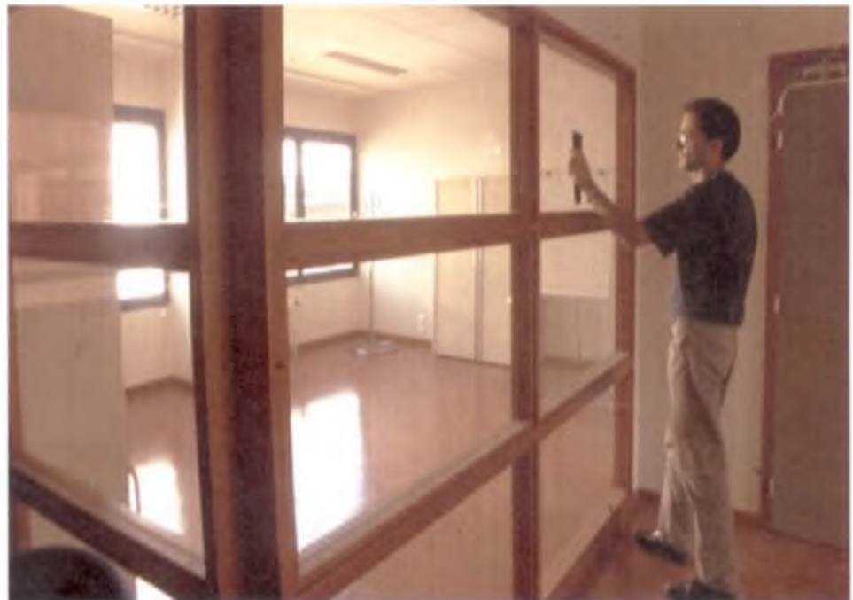
Δ Under standard sky conditions adjusted for a horizontal external illuminance of 10,000 lux, the luminous flux entering the space can be computed by multiplying the illuminance behind the windows by the area of the glazing. This leads to comparison of the performance of various daylighting systems in terms of lumens brought to the space.
