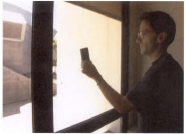
Δ Assessment of hemispherical - hemispherical transmittance of diffusing awnings. No direct sun beams should hit the window pane - overcast sky conditions preferred.
