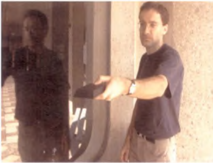
Δ Determination of the contribution of light reflections on the external ground. The luxmeter is oriented upward and downward to compare light coming from the upper and lower hemispheres.
