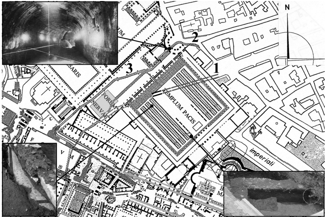
Fig. 4 Before the Templum Pacis . Top-left inset: the Cloaca Maxima (from Bauer 1983, pl. 62.1: 1, 2, and 3 indicate the main phases of the cloaca). Bottom-left inset: mosaic floor of a Republican house (from Capponi, Ghilardi 2001, fig. 5). Bottom-right corner: wall in opus incertum with lead pipe (in the circle) excavated in July 1999 (photo author).
