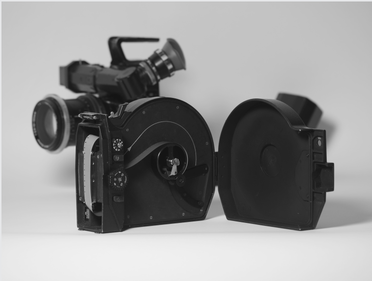
Figure 1.5 The 400ft coaxial magazine of the Arriflex SR, showing the take-up side of the magazine. Camera courtesy of The New School Film Office.
