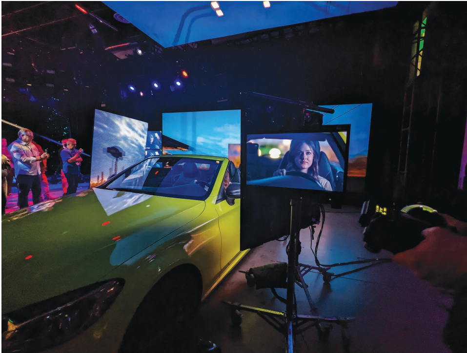
Figure 1.5 An LED volume displays a moving environment while a stationary prop car is manipulated by an actress Source: (Image courtesy of PRG)
