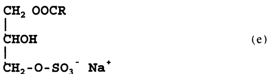
FIG. 9 Sulfate esters: examples of sodium salts derived from (a) fatty alcohol; (b) fatty alcohol ethoxylate; (c) fatty acid alkanolamide; (d) alkylphenol ethoxylate; (e) fatty acid monoglyceride.
