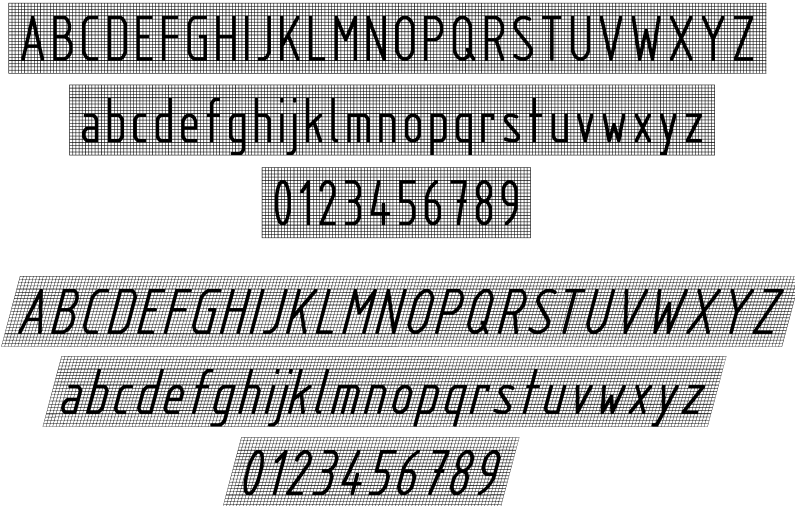
Figure 2.16 Lettering style A (vertical and italic) according to ISO 3098.
