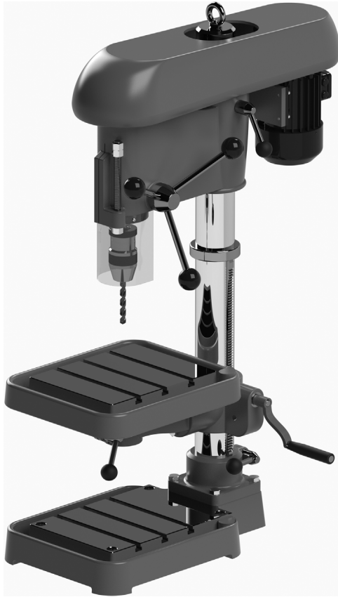
Figure 1.5 Rendered CAD model of a pillar drill.
