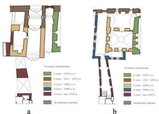
Figure 5. Diagram of the periods of construction of the Church of the Exaltation. a) First floor, b) Second floor. The author's drawing.
