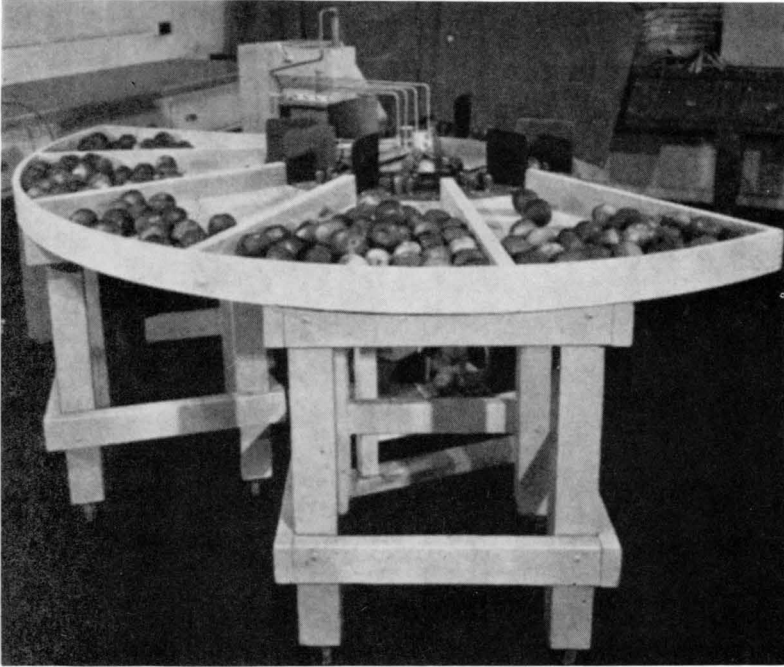
Figure 1.11 An experimental fruit sorting machine employing principles of light transmittance (Yeatman and Norris, 1965)
