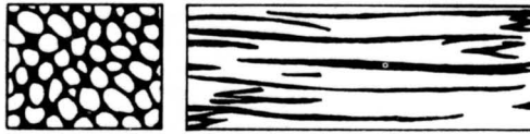
Figure 2.7 Fibrillar structure of natural cellulose fibre; dark regions represent intercellular spaces (Meredith, 1956)
