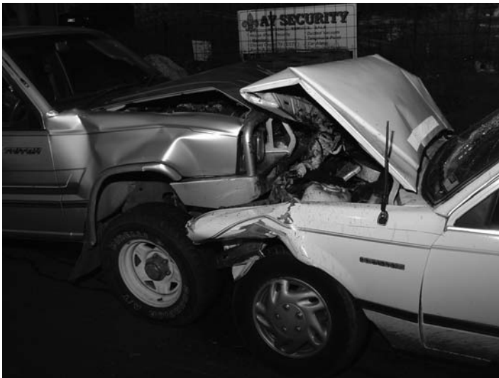
Figure 1.3 Frontal collision of passenger sedan and four-wheel drive vehicle showing override.
