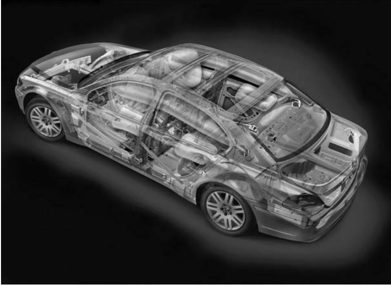
Figure 1.2 Longitudinal and transverse components of body shell. (Drawing courtesy of BMW.)
