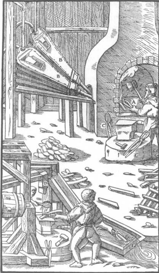
3. A smithy, as illustrated in Georgius Agricola, De re metallica (Basel, 1556). The scene would have been little different in Richard of Wallingford's day, although the bellows here ( B ) are rather grand, and like the trip hammer ( D ) water-powered, something unlikely in the Wallingford smithy. The forge ( A ), the tongs and anvil ( C ) and the quenching water ( E ) would have been familiar, as would the boys, with their leather aprons.
