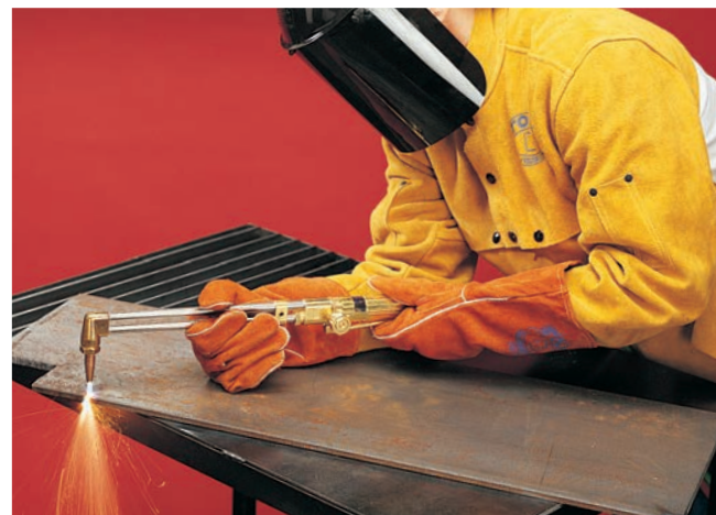
Oxyacetylene cutting (OAC).
