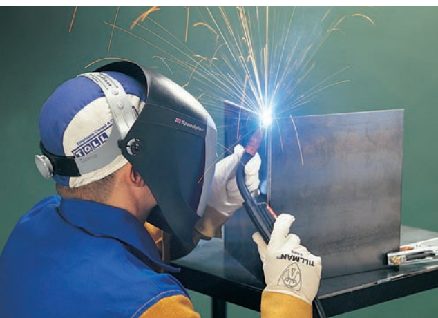
Gas metal arc welding (GMAW).
