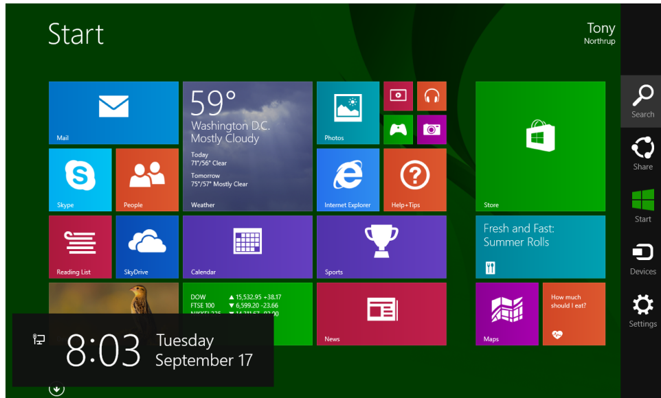
Figure 1-10 Use charms to access settings and functions you might have used menus to access in earlier versions of Windows.
