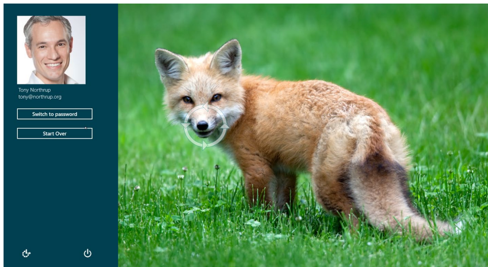
Figure 1-18 Draw lines, dots, and circles (as shown around the fox’s nose) to log in using a picture password.
