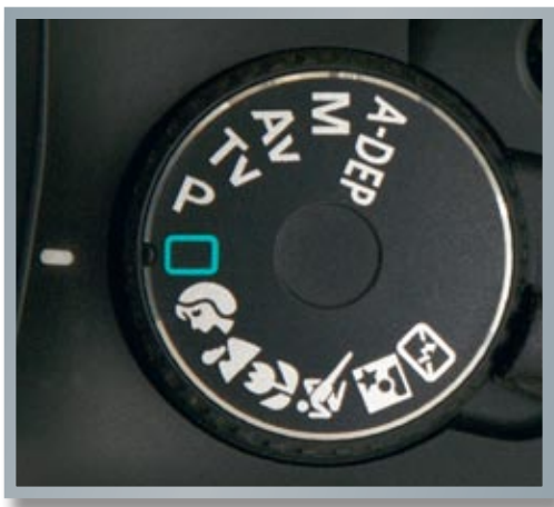
Set the camera's Mode dial to the green box to select Full Auto mode.
