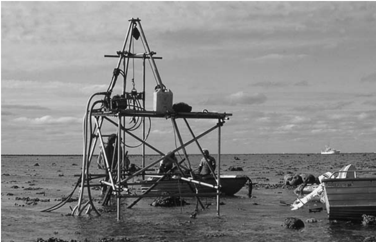
Figure 1.4 The James Cook University hydraulic drilling rig on Gable Reef typical of the equipment used during the 1970s onwards to obtain cores through the reef to about 30 m.
