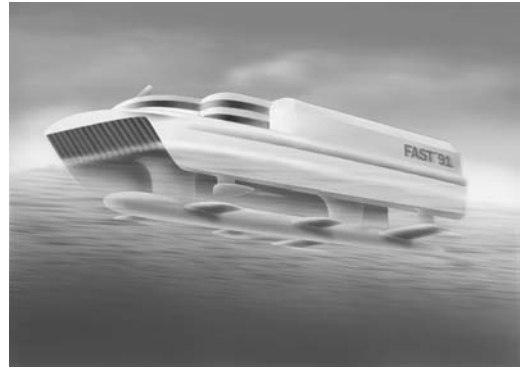
Figure 1.1. Fictitious high-speed vessel with air cushion, foils, and SWATH effects. (Artist: Bjarne Stenberg)
