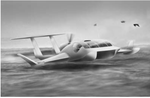
Figure 1.11. Artist's impression of a WIG vehicle based on the Hoverwing technology by Fischer-Flugmechanik. An air-cushion effect is generated between the floats during takeoff. (Artist: Bjarne Stenberg)
