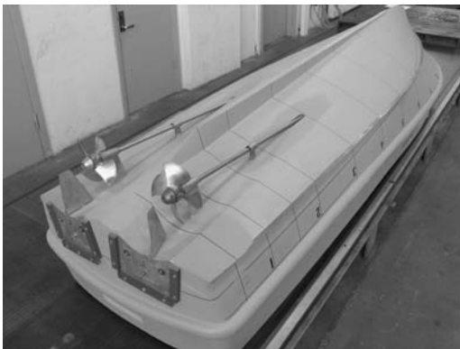
Figure 2.2. Propellers with inclined shafts installed on a model of a planing vessel with hard chines. Propeller tunnels are used to minimize the shaft angle. The rudders are twisted and adapted to the propeller slip stream. Two interceptors are placed at the transom to control the trim angle (see section 7.1.3 and Figure 7.5 for more details about interceptors). (Photo by K.A. Hegstad)
