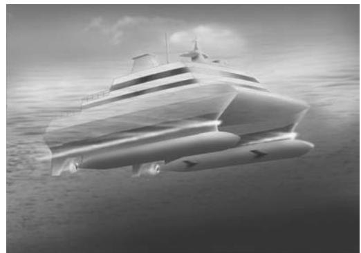
Figure 1.2. SWATH (small waterplane area twin hull). (Artist: Bjarne Stenberg)
