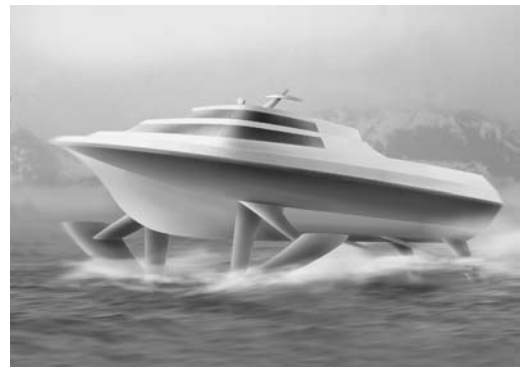
Figure 1.7. Hydrofoil vessel with free surface–piercing foils. (Artist: Bjarne Stenberg)
