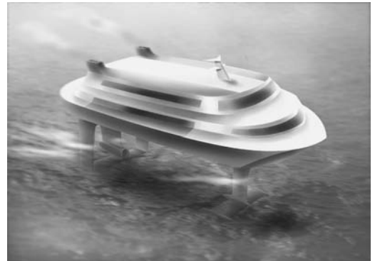
Figure 1.6. Hydrofoil vessel with fully submerged foil system. (Artist: Bjarne Stenberg)
