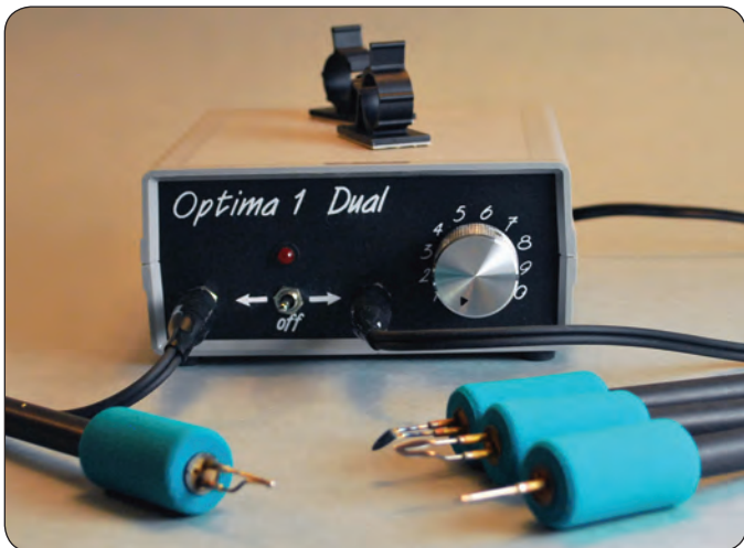
Figure 1.5. This variable-temperature unit is set up to run two burning pens at the same time. The on/off switch allows you to move easily from one pen profile to another with little effort. The temperature range for this unit is far greater than the temperatures needed for burning wood, gourds, paper, and leather. This particular manufacturer also offers several options, including high-voltage cords, and extra-thick wire pen tips for added strength.
