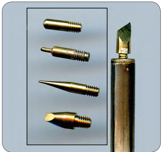
Figure 1.3. One-temperature tools use interchangeable brass tips that screw into the shaft of the pen. Note that the tip of the pen has been left slightly open to show the threading. Five pen styles are available, and these can be used for the projects. The pen is shown with the universal tip, which creates fine lines and wide shading strokes. From top to bottom on the left are the wide ball tip, the medium ball tip, the micro-ball tip, and the square lettering tip.
