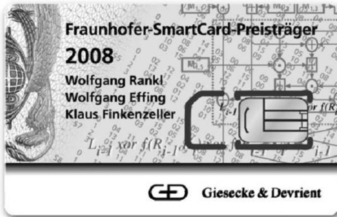
Figure 3.47 A smart card with a special module for direct connection to a PC. Its four contacts have the same form as a USB plug. After the card is broken free from its carrier and placed in an adapter, it can be plugged into the USB port of a computer. This arrangement allows smart card technology to be used directly with computers, without using an intermediate terminal (Reproduced with permission from Giesecke & Devrient)
