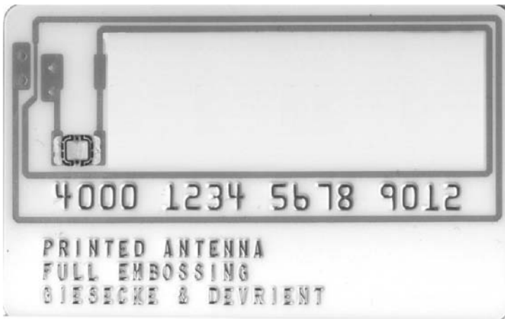
Figure 3.25 An example of a credit card with embossing and an antenna for contactless communication. This is a functional sample without issuer-specific printing (Reproduced with permission from Giesecke & Devrient)
