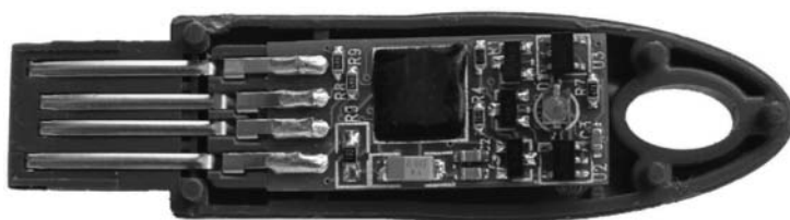
Figure 3.13 Example of an alternative smart card form factor. This photo shows a USB plug with a soldered-in smart card microcontroller and the necessary interface components, which has been opened up to reveal its internal components
