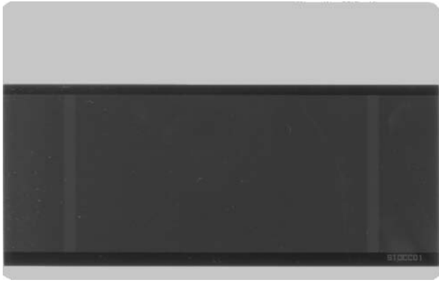
Figure 2.15 A typical optical memory card with a net storage capacity (including error correction) of approximately 4 MB. The raw storage capacity (without error correction) is approximately 6 MB
