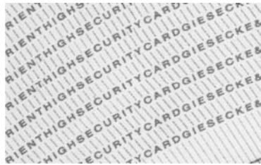
Figure 3.23 A highly enlarged example of microtext, which cannot be printed using ordinary commercial printing processes (Reproduced with permission from Giesecke & Devrient)
