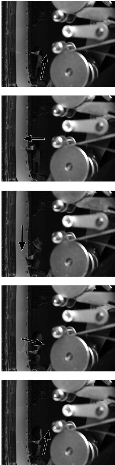
Figure 1.1 I: The pulldown claw of a non-reflex Bolex H16 camera with the pressure plate removed to better see the sequence of actions of the claw. The arrows indicate the movement of the claw as it advances the film between exposures, and then retracts, moving back into position during the exposure of the film.
