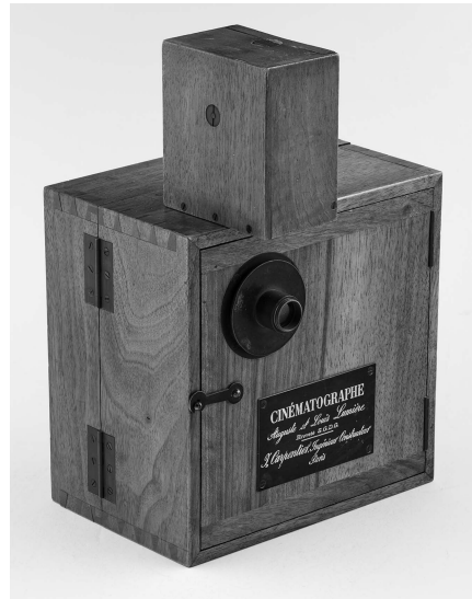
Figure 1.2 The Lumière’s cinématographe 35mm hand-crank motion picture camera. In the words of Erik Barnouw: “The cinématographe could be carried as easily as a small suitcase.” Courtesy of the George Eastman Museum.
