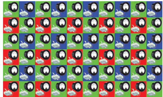
Figure 1.30 A Bayer pattern sensor is comprised of rows of red, green, and blue filtered photosites.
