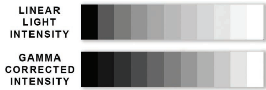
Figure 1.14 Linear light intensity visually compared to gamma corrected intensity.
