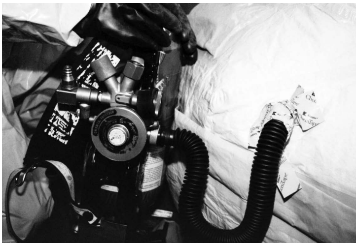
Figure 5.3 The primary purpose of the RIT is to provide an emergency air supply for personnel in Level “A” protective clothing who become disabled during an entry until they can be extricated.
