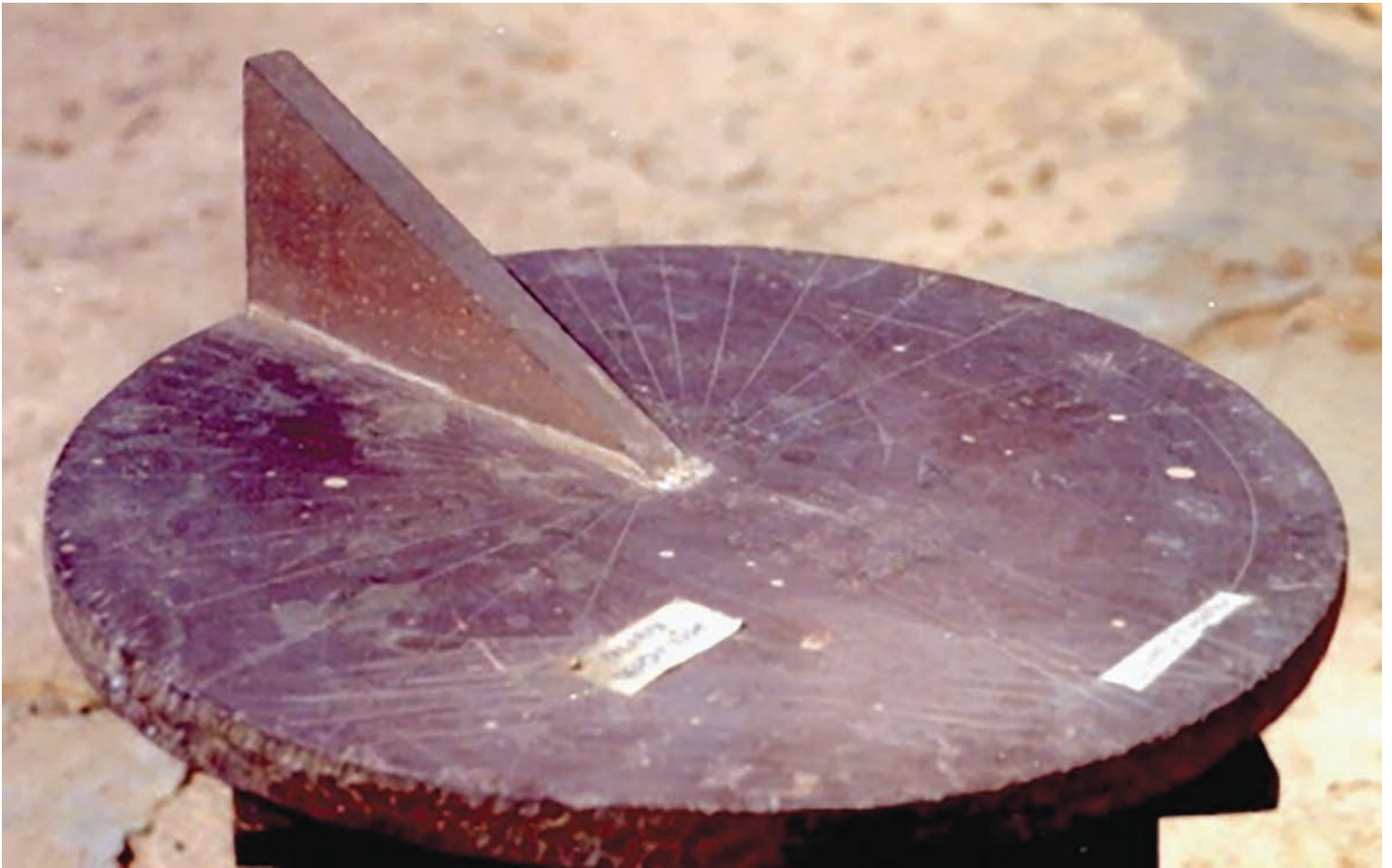
Figure 10 Palabhā-yantra made by Gokula Nātha Śarmā in 1882, Jai Singh Observatory, Jaipur. Photo: S. R. Sarma.
