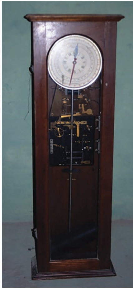
Figure 14 Synchronome clock with a dial for hours and ghaṭīs . Photos: S. R. Sarma.
