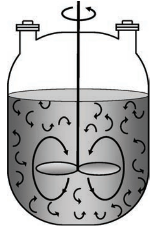
Figure 1-5(b) Batch reactor mixing patterns. Further descriptions and photos of the batch reactors can be found in both the Visual Encyclopedia of Equipment and in the Professional Reference Shelf on the CRE Web site.
