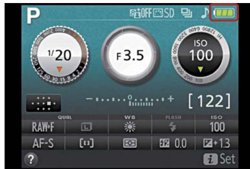
Figure 1.1 The LCD screen shows how much charge is left on your battery.
