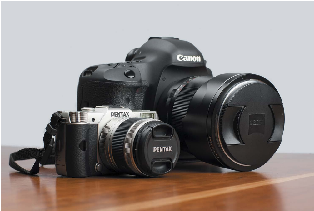
Figure 1.4 To get a sense of size difference between various DSLRs, check out this full-frame DSLR Canon body next to a Micro Four Thirds Pentax body, both with lenses.
