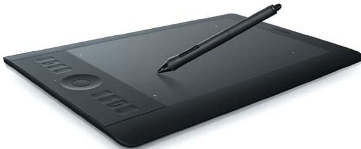
1.6 A digital tablet permits additional accuracy and prevents wrist strain.
