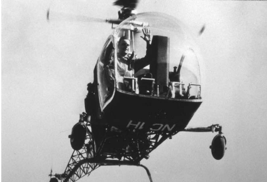
Fig. 1.6 The legendary Bell 47 was based on Arthur Young's research and was the first helicopter to be certified in the USA. Larry Bell never liked the utilitarian appearance, but it outsold all of the more stylish models. The flybar stabilization system was adopted extensively in later Bell machines. (Bell Helicopter Textron)
