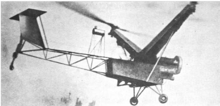
Fig. 1.2 The Weir W-5 flew extensively, but development of all helicopters was suspended in the UK during World War II. (AugustaWestland)
