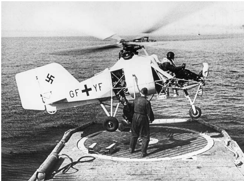
Fig. 1.4 The Flettner Kolibri (Hummingbird) was the first synchropter and was an advanced and capable machine. Kaman developed the concept and produced the successful Husky and K-Max models. (Steve Coates)
