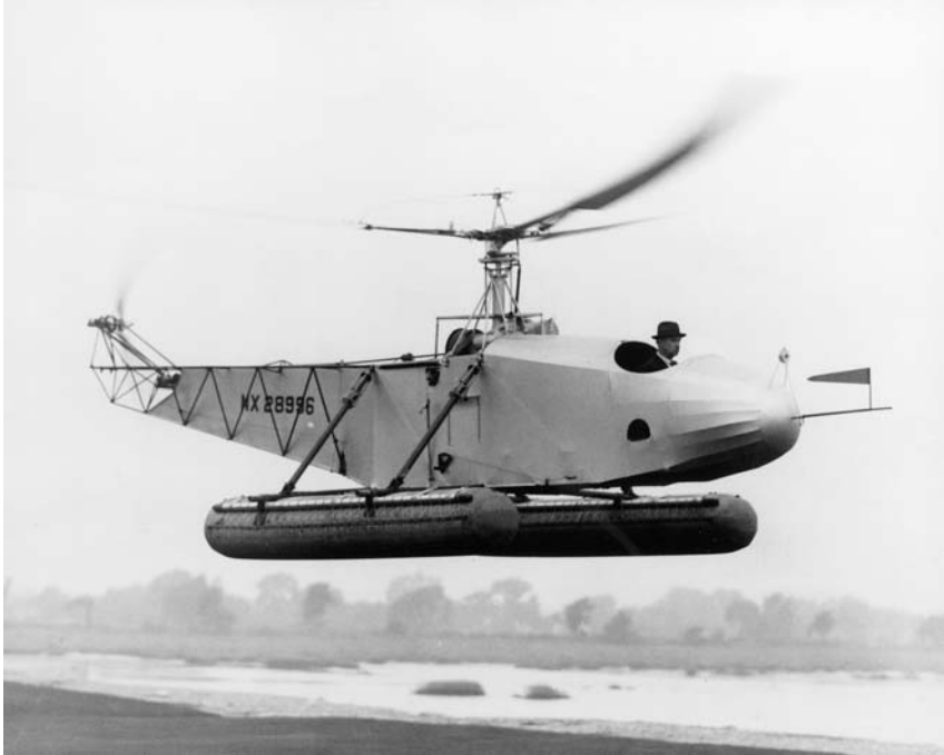
Fig. 1.3 The Sikorsky VS-300 had an extended development period during most of which cyclic control was not understood and unwieldy auxiliary rotors were used instead. (Igor I. Sikorsky Historical Archives Inc.)
